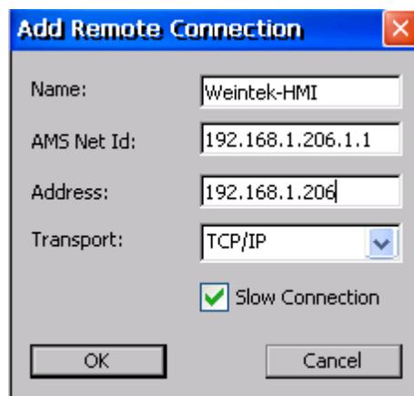
h. Return to Control Panel; execute CX Configuration Tool to confirm PLC AMS Net Id.
